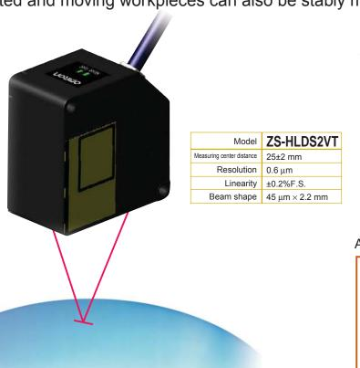
A special aspherical lens was developed for the ZS-HLDS2VT, and the design of the optical structure was optimized for regular-reflective workpieces. This has greatly increased the allowable degree of tilt and improved stability for measuring transparent and regular-reflective workpieces.
