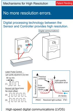
used between Sensor and Controller. Image signal stabilizes because the clock error between the control signal from the Controller and the light reception device disappears. Optimum light quantity adjustment is possible with laser power algorithms that can be adjusted to any level, which facilitates super high resolution.
